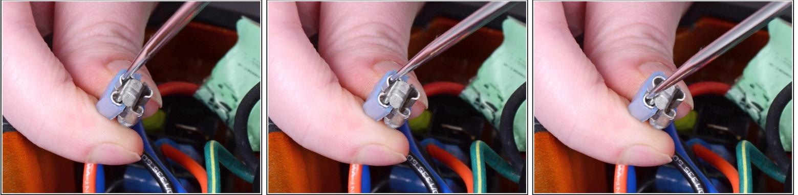
⚠ Be **very** careful with this connection, as even minimal bending can break the metal conductor [in half](#).
