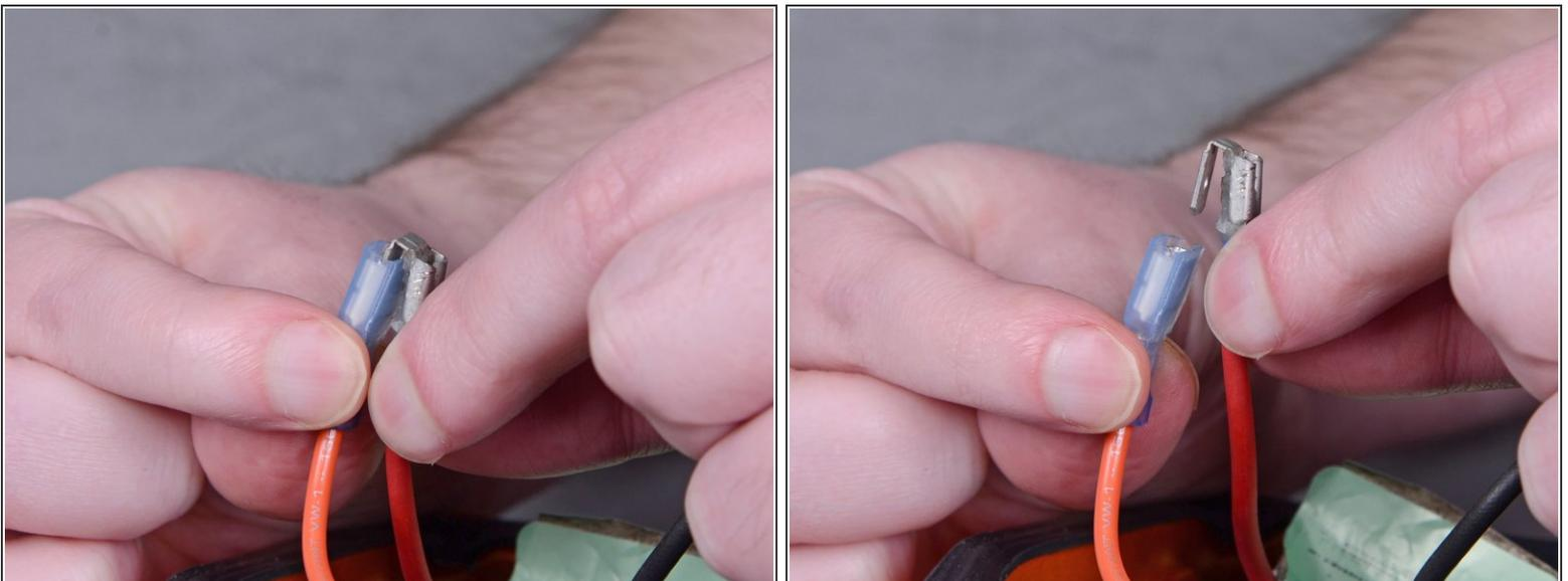
⚠ Be **very** careful with this connection, as even minimal bending can break the metal conductor [in half](#).
