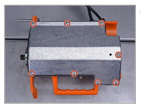
• Remove the eight Phillips #2 screws on the underside of the cutting head.
