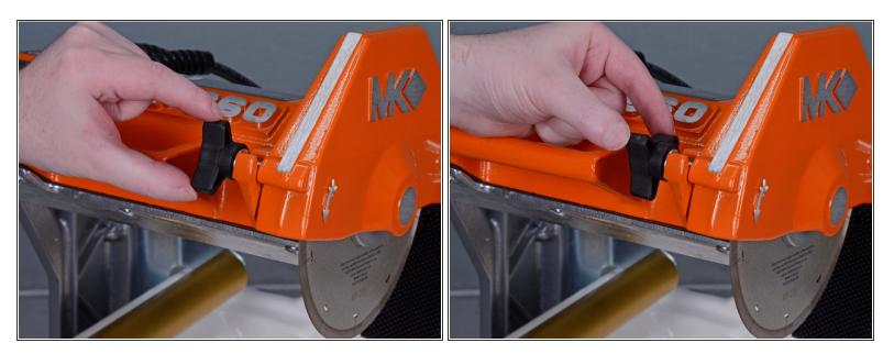
• Loosen the plastic knob holding the blade cover in place.
