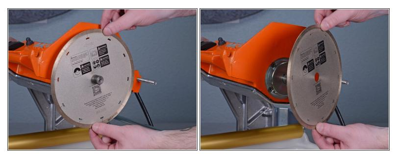
• Remove the cutting blade.
