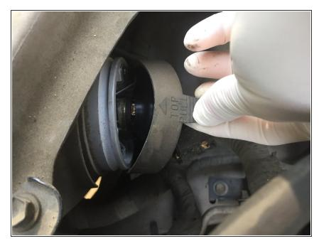
Pull out the rubber cover. If maintenance is not done often on the car the rubber cover may get stuck. This can be solved by using tools to push or pry out the rubber cover.
