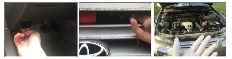
Pull the hood lever to unlock the car hood. Pull the safety lever upwards and push the hood of the car open. Put the hood strut (metal rod) to hold the hood up.
