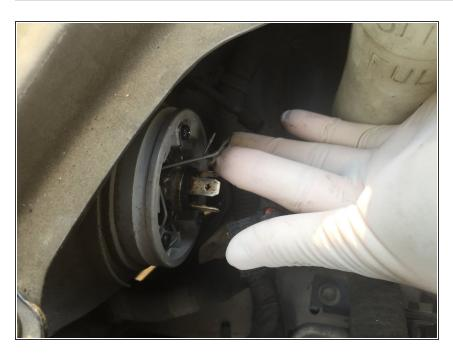
Unhook the metal clip fixing the unusable lightbulb.
