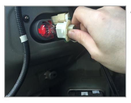
Remove the bulb assembly (twist counterclockwise). The light bulb assembly is located above the center of where the plastic cover (before it was removed).
