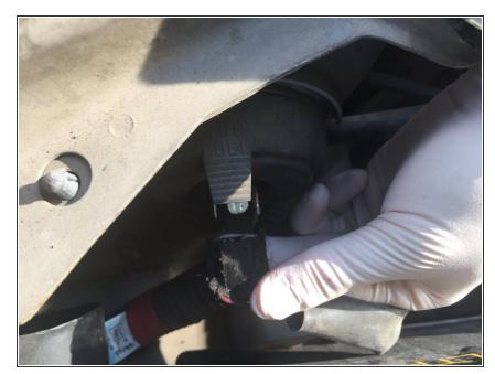
Remove the connector (wire)
