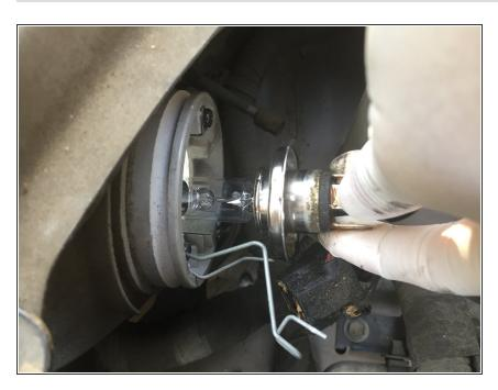
Remove the unusable light bulb and place in the new light bulb.
