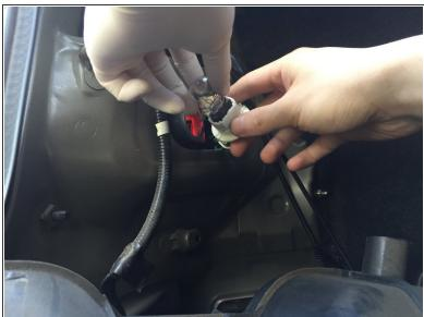
Pull the light bulb from the socket.
