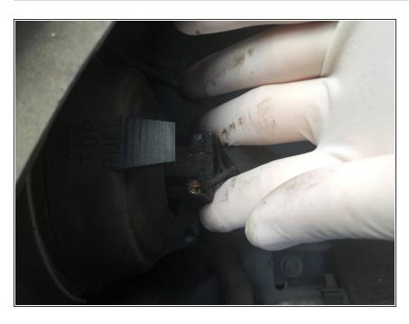
Plug the connector into the new light bulb.
