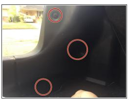
Open the trunk of the car. Remove the 3 screws on the plastic cover using the Phillips #2 screwdriver. All of them will the same length of 19.0 mm, and will not have to be put in back into the exact same positions.
