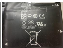
Lift the battery out of the case vertically
