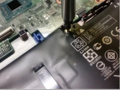
Remove 4x PH-0 Philips head 3mm screws (circled)
