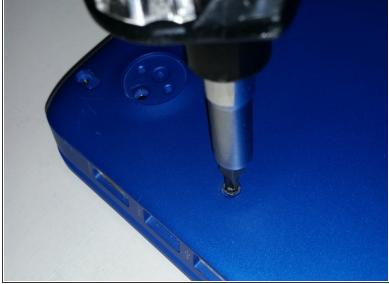
Remove the 11x 5mm Phillips PH-0 screws (circled)
