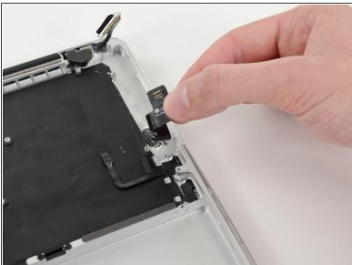
Lift and remove the headphone jack out of the upper case.
