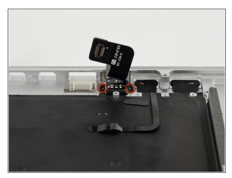
Remove the two 3.4 mm T5 Torx screws securing the headphone jack to the upper case.
