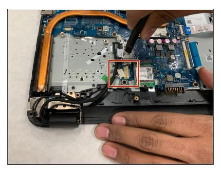
Use a spudger to disconnect the power cable from the motherboard.
