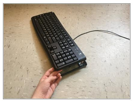
• Remove the top of the keyboard and put it aside.
