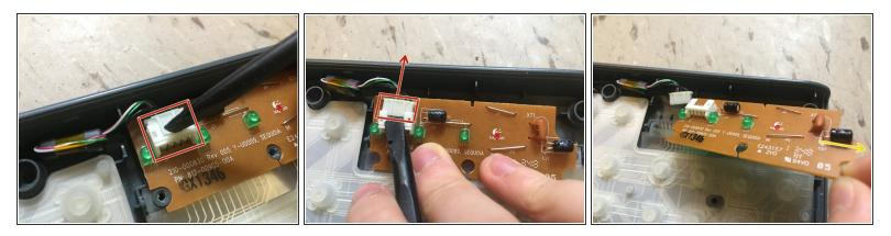
• Use the spudger and carefully pry the connector out of its socket. (Highlighted in the pictures)
