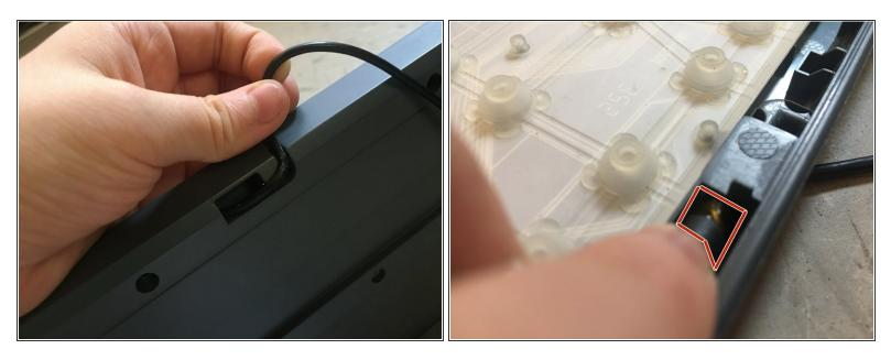
• Carefully nudge the connector out of the hole in which the cable enters the keyboard's chassis.
