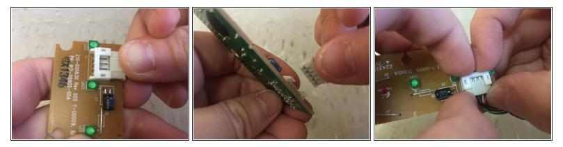
• Connect The Cable To The Circuit Board.
