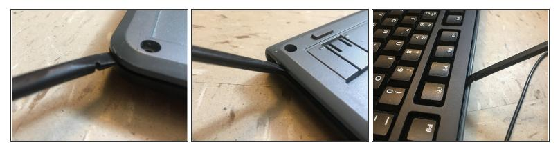
• Use the spudger to separate the top of keyboard from the bottom of the keyboard.
