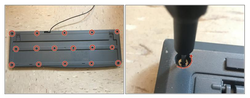
• Remove the Phillips #000 screw. Turn the screwdriver counter-clockwise.
