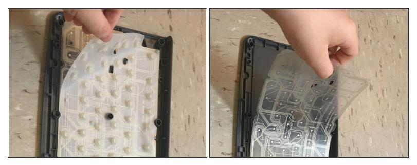
• Peel the membrane off carefully so that the membrane doesn't rip.
