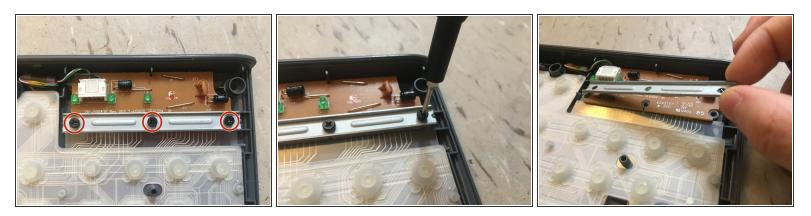
Unscrew the highlighted screws using a Phillips #000 Screwdriver. Turn the screwdriver counterclockwise.
