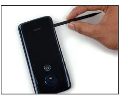
Insert a spudger into the lower half of the left side of the phone about 2 cm and slide it down
