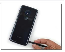
• Insert the flat end of a spudger into the lower half of the right side of the phone about 2 cm and slide it down the right edge to release the right strip of adhesive.
