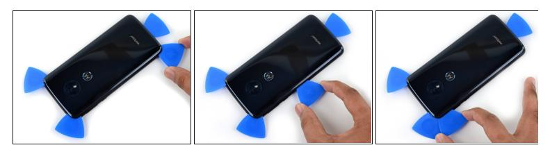
• Slide a pick along the left edge of the phone to slice through the rear glass adhesive.
