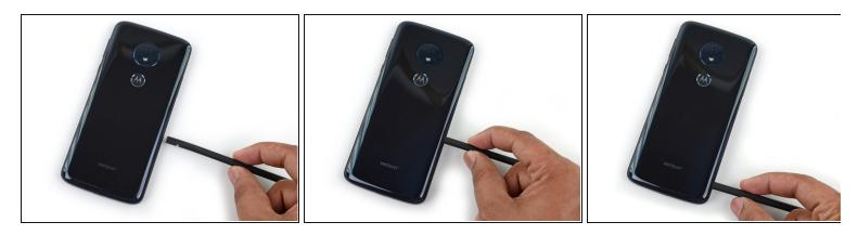
Insert the flat end of a spudger into the lower half of the right side of the phone about 2 cm and slide it down the right edge to release the right strip of adhesive.
