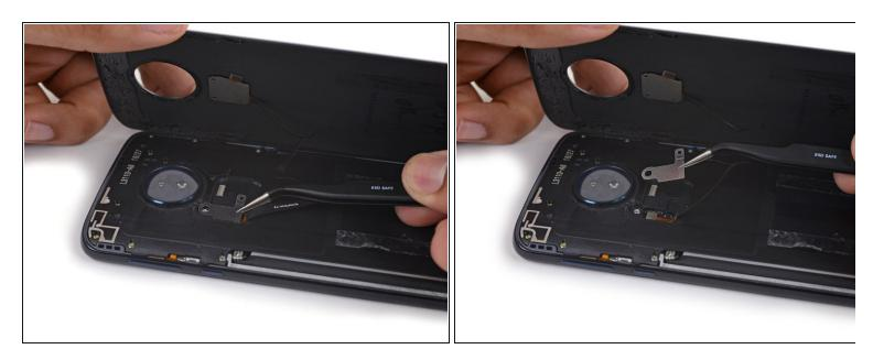
• Use a pair of tweezers to remove the fingerprint sensor cable retention bracket.
