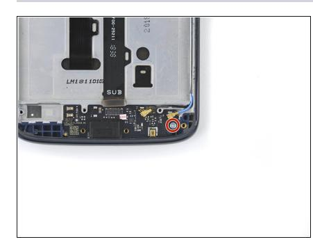
Use a Phillips screwdriver to remove the single silver 2 mm screw securing the daughterboard.
