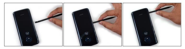
• Insert a spudger into the lower half of the left side of the phone about 2 cm and slide it down the left edge to release the left strip of adhesive.
