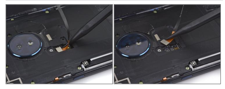
• Use the pointed edge of a spudger to disconnect the fingerprint sensor cable.
