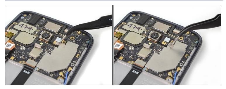
Use a pair of tweezers to carefully remove the tape covering the camera module connector.
