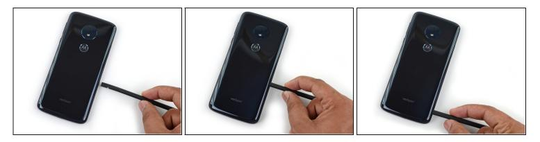
• Insert the flat end of a spudger into the lower half of the right side of the phone about 2 cm and slide it down the right edge to release the right strip of adhesive.
