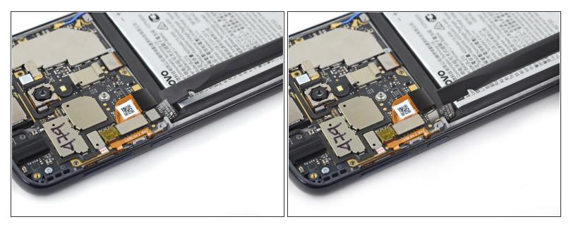
• Use a spudger to pry up and disconnect the battery cable.
