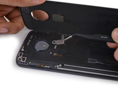
• Use a pair of tweezers to remove the fingerprint sensor cable retention bracket.
