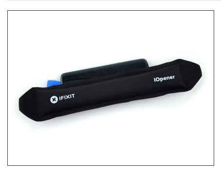
Heat the right edge of the back of the phone to soften the adhesive underneath.
