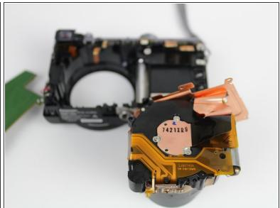
Lift the camera lens from the camera.
