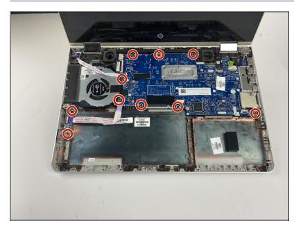
• Remove ten 4 mm screws using a Phillips #00 screwdriver.
