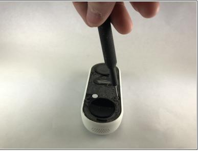
Peel back the cover stickers and use the Phillips #000 screwdriver to remove the four screws.
