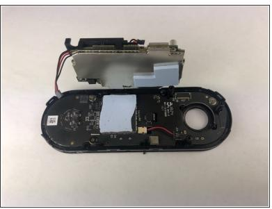
Holding the device as shown push the circuit board away from you and up to free it from the clips.
