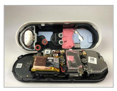
Use the Phillips #000 to remove the two screws holding the ribbon cable to the white casing.
