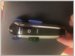
• Unclip the black cover, using a slim tool like an iSesamo or with some guitar picks. Insert the tool alongside the gap between the two pieces.
