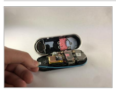
Remove the O-Ring (colored blue) from the device. It is placed around the edge of the motherboard.
