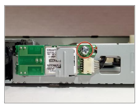
Use a Phillips #1 screwdriver to remove the single 5mm screw that holds Wi-Fi module to the device.
