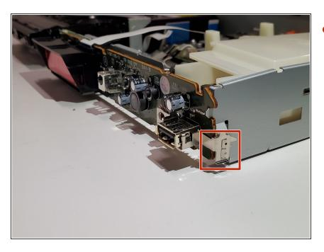
Unclip the metal piece on the lower right corner by gently lifting it up.
