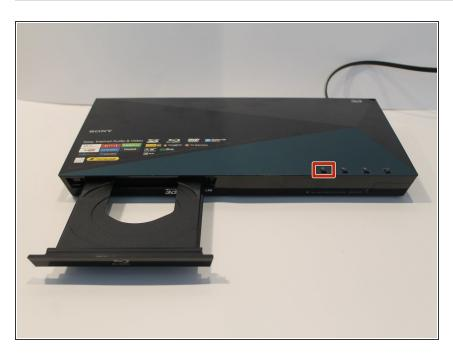
Plug in the device to turn it on, then press the eject ( ) button to open the tray.
