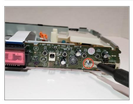
Using the Phillips #1 screwdriver, remove the 5mm screwdriver attached to the port board.
