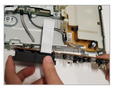
Remove the port board by simply pulling it away from the device.
