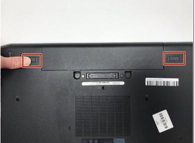
Slide the switches away from each other to release the battery.
