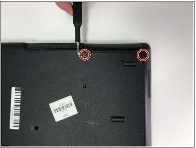
Using a Phillips #00 screwdriver, unscrew the two screws.
