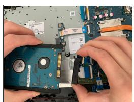
Remove the data connector from the hard drive.
