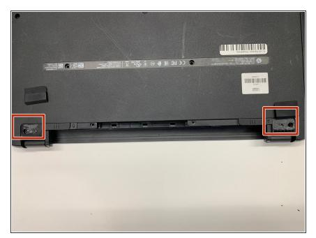
Remove the two rubber feet next to the battery.
