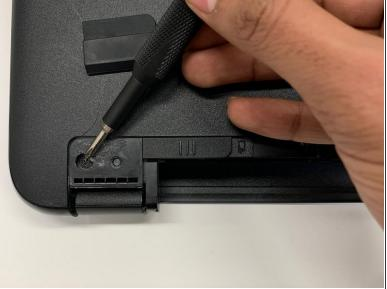
• Remove twelve 8mm Phillips #00 screws including two underneath the rubber feet.
