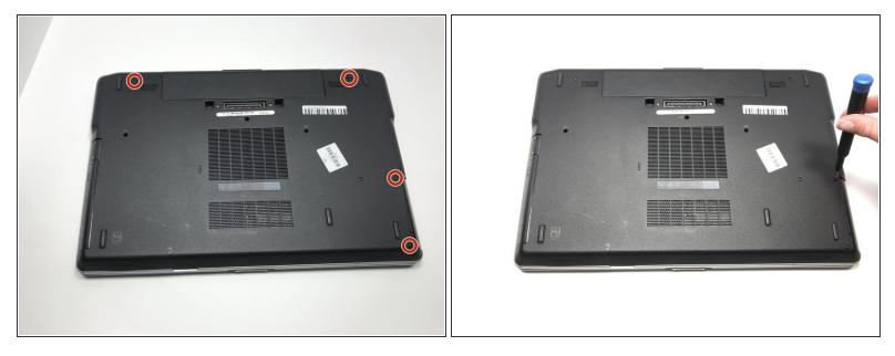
• Remove the four screws to remove the back panel using the Phillips #00 screwdriver.
