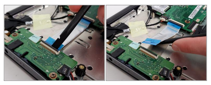
Use a spudger to carefully disconnect the ribbon connector from the right side of the sound card.
