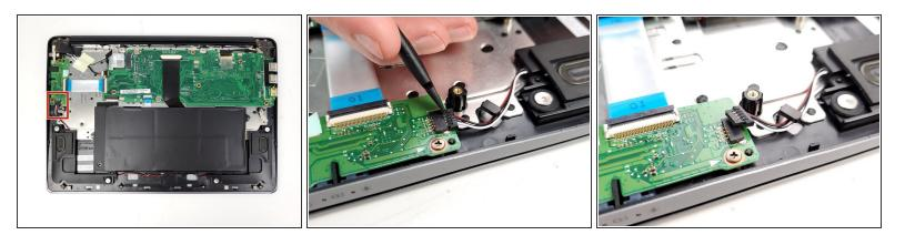
Use a spudger to disconnect the speaker connector from the bottom of the sound card. The connector should slide out toward the left speaker's housing.
