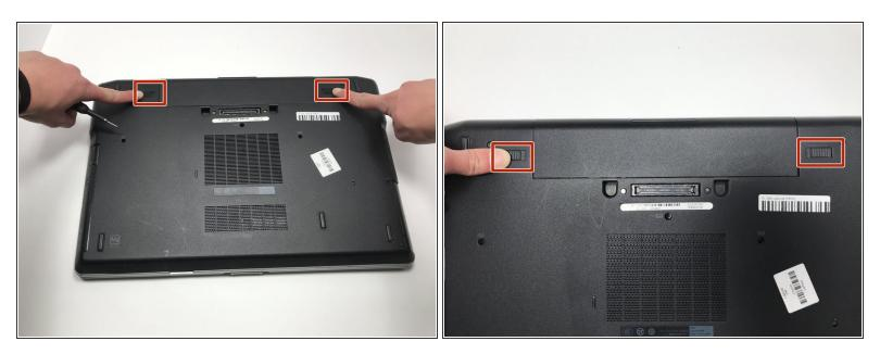
Slide the switches away from each other to release the battery.
