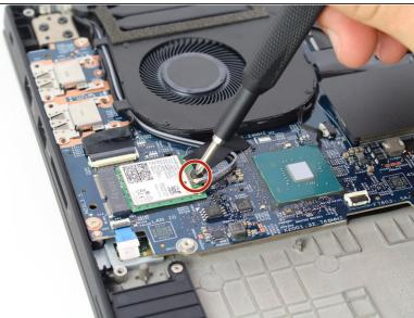
Using a Phillips #00 head screwdriver, remove the 3mm screw holding the wireless adapter to the motherboard.
