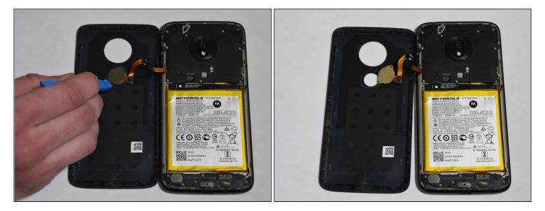
• Use the iFixit pick and the iFixit opening tool to pull the fingerprint scanner off of the back case.
