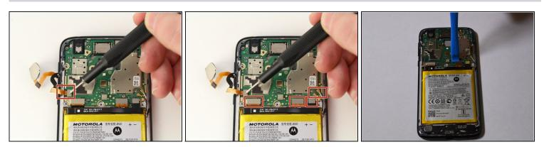
• Using an iFixit opener tool, detach the fingerprint sensor and the other 5 cables from the motherboard.
