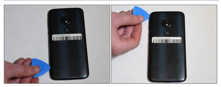
• Use the iFixit pick to break the adhesive around the back case.
