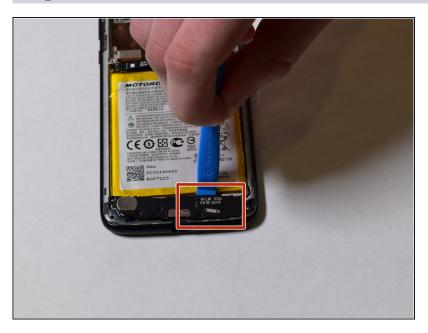
• Using the iFixit opening tool, carefully pry up the charging port assembly cover.
