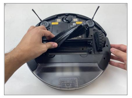
Pull the main brush slightly to the right to remove it from the compartment.
