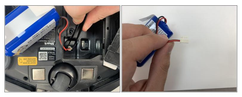
A Be careful when removing the connector, as the part can break if too much force is used.
