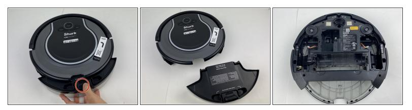
• Push down on the black tab and remove the dust bin
