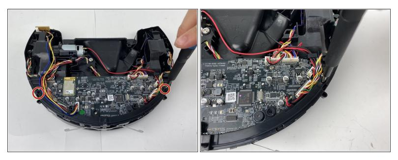
(i) Make sure that both the left and right side sensors have been removed from their compartments.
