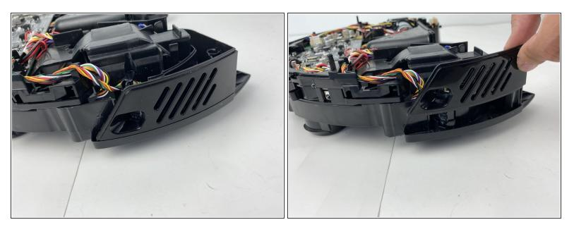
• Lift up the diagonally vented cover on the side of the robot containing the side sensor.
