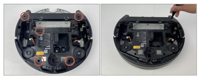
Using a Torx TR15 screwdriver, remove the five screws from the bottom cover.
