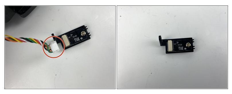
Disconnect the white connector from the sensor.
