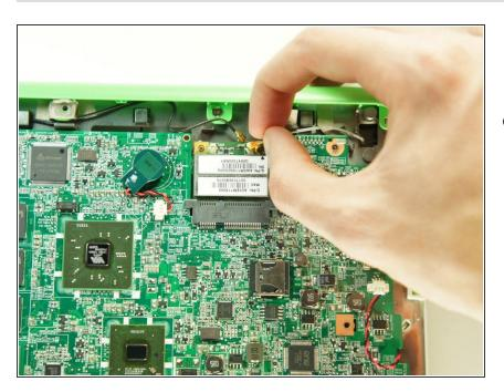
Gently remove the two antenna cables by lightly pulling the cable connectors up.
