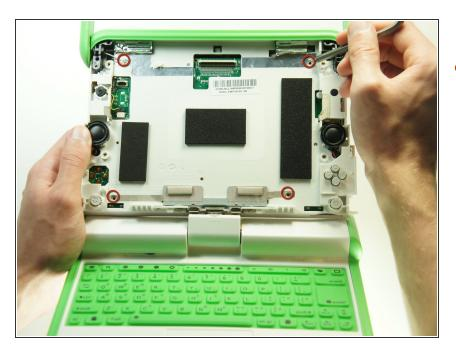
Remove the four 4mm Phillips #1 screws that hold the top cover to the case.
