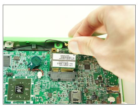
• Remove the wireless card by gently lifting it out of the socket.
