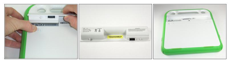
• Lift the middle of the battery to remove it.
