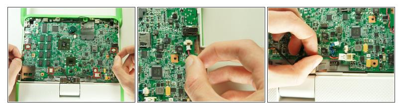
Disconnect the five cables that connect the motherboard to the case by pulling them straight out of their sockets.
