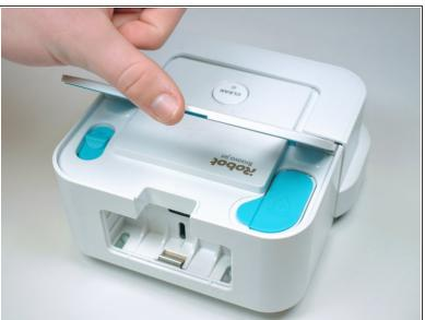
Lift up the handle to reveal the eject button.
