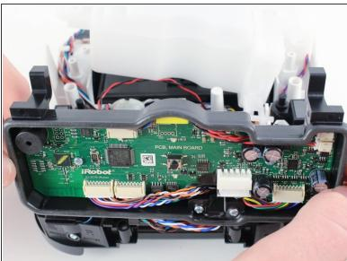
• Lift up on the motherboard case to remove it from the device. This will expose the water tube that is attached to the tank.
