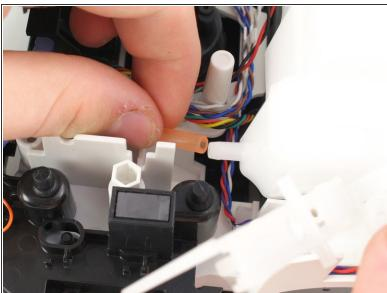
Pull the tubing off of the tank connector.
