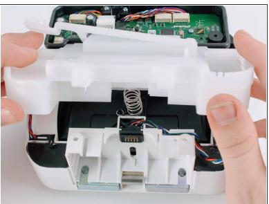
Lift the tank up and away from the device.
