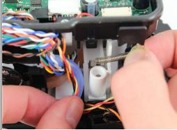
First pull up, then pull down on the spring to detach it from the hooks.
