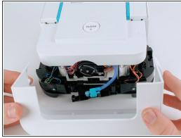
Carefully pull back on the front shell to remove it from the robot.
