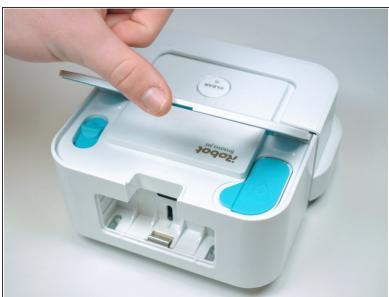
Lift the handle to access the filter.
