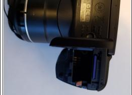
Remove the battery located at the bottom of the device.
