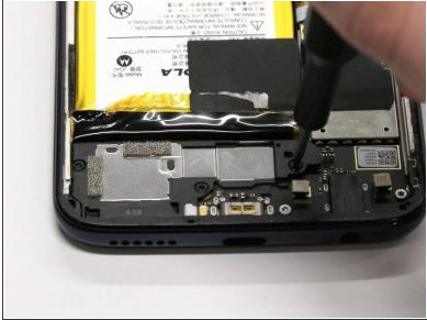
• Use the Torx T5 screwdriver to remove the three 3.0 mm screws.
