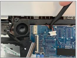
Using the curved end of the Halberd Spudger, disconnect the Speaker Cable from the port that connects it to the motherboard. To complete this step, use the curved end of the spudger to pry the plug out of the port.
