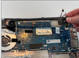
Using the thin end of the iFixit Plastic Opening Tool, pry the speakers out of their place inside the laptop's base.
