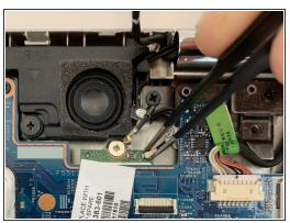
Use the Blunt Tweezers to disconnect the Wireless Card Antenna Cables. Start with the cable labeled M2, which is connected to Port #2. To disconnect he cable, grab it on both sides with the tweezers and pull up.
