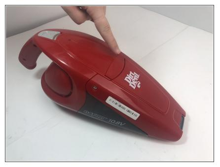
• Press the button found in the middle of the vacuum downwards. Then, separate the front from the back of the device by gently pulling apart.
