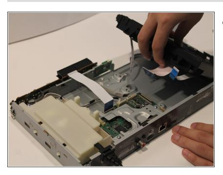
Remove the metal brace then remove the disk tray.
