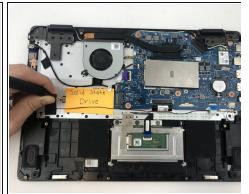
Using a Phillips #1 screwdriver, remove the one 4mm screw that secures the Solid State Drive.
