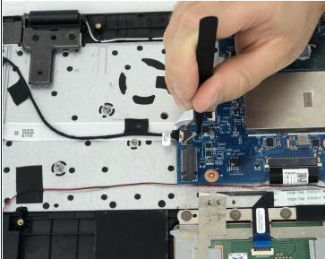
Using the tweezers, pull the black CQWP connection wire from its port.
