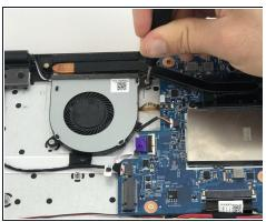
• Use Phillips #1 screwdriver to remove the two 4mm screws that are securing the fan.
