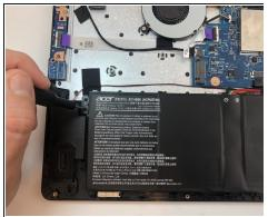
• Use a Phillips #1 screwdriver to remove two 4 mm screws that secure the battery.
