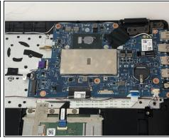
• Use the tweezers to disconnect the wiring harness in the bottom right corner of your laptop.
