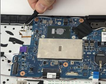
• Using the tweezers, pull out the orange GND VCC connection wire.
