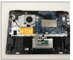
Grasp the CMOS battery with the tweezers and remove it from the motherboard.
