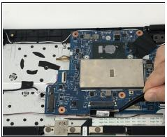
• Using the tweezers, remove the black drift cable from its port.
