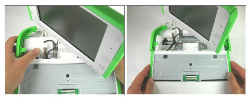
Rotate the entire lower assembly up slightly, and pull it away from the screen to free it from the screen hinge.
