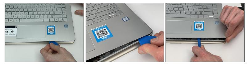
Using the iFixit Plastic Opening Tool and the iFixit Opening Picks, work your way around the rest
