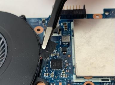
Using the Metal Tweezers, pull up the tape connecting the fan connector to the motherboard.
