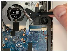
• Using the plastic Spudger, remove the ZIF connector that connects the motherboard to the Display Cable. To remove a ZIF connector, use the flat end of the Spudger to flip up the cap on the top. Then the connector should slide out.
