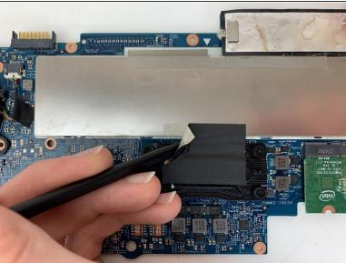
Using the flat end of a plastic Spudger, peel back the tape located on the bottom of the motherboard between the heat sink and the motherboard.
