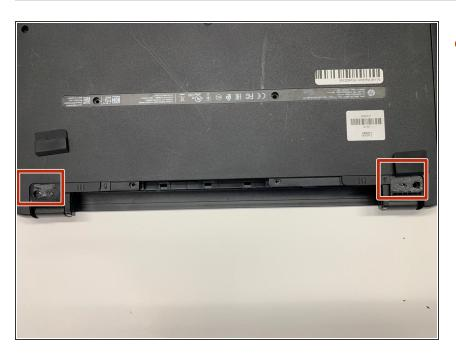
Remove the two rubber feet next to the battery.
