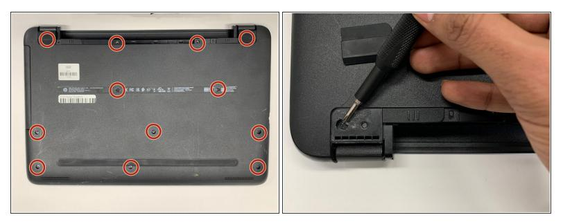
Remove twelve 8mm Phillips #00 screws including two underneath the rubber feet.
