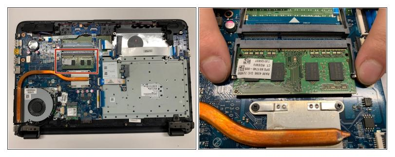
• To release the RAM, hold and pull the strips outwards on either side of the RAM.
