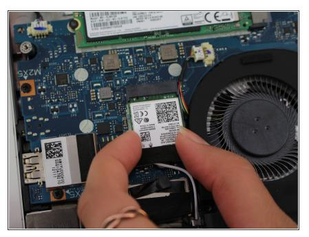
Grab the adapter from both sides and pull towards the hinge to remove the adapter from the device.
