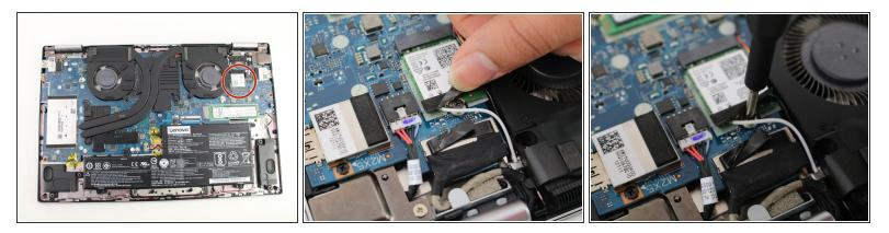
• Lift the foam covering the connecting wires and screw, and use the Phillips #0 screwdriver to remove the 2mm screw.
