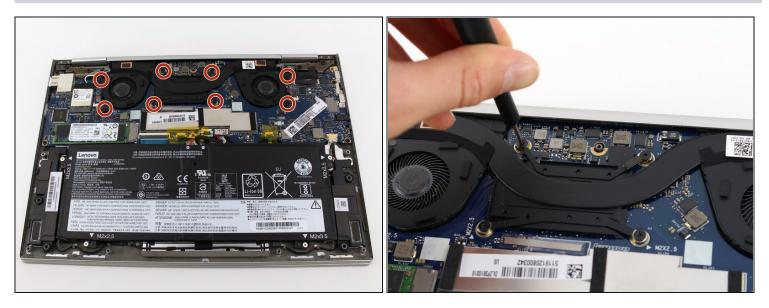
• Use a Phillips #00 screwdriver to remove the eight 2.5mm screws securing the heat sink assembly.
