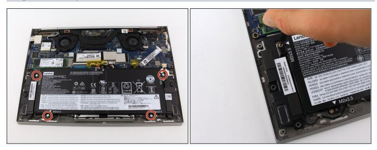
• Remove the four 3.5mm Phillips #0 screws securing the battery.
