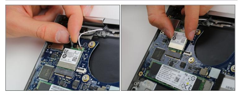
• Gently slide the LAN card straight out of the motherboard connector.
