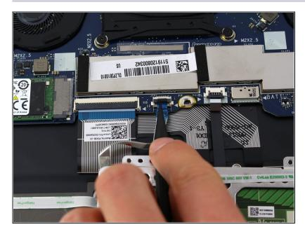
• Use a spudger to remove the fingerprint sensor cable by flipping up the gray connector tab. Pull out the cable.
