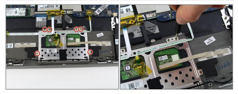
• Use a Phillips #00 screwdriver to remove the six 2.5mm screws holding down the touch pad.
