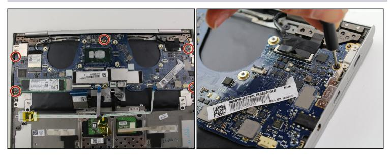
• Use a Phillips #00 screwdriver to remove the five 3.5mm screws securing the motherboard.
