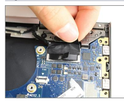
Peel back the adhesive cover connecting the display connector and hinge.
