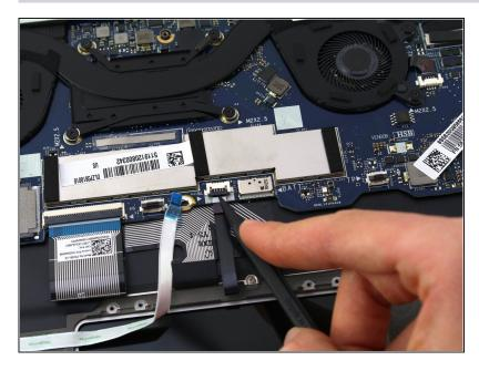
• Use a spudger to remove the bluetooth cable by flipping up the gray connector tab. Pull out the cable.
