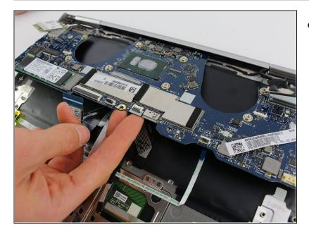
• Remove the motherboard by holding it by the bottom and pulling diagonally away from the laptop.
