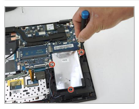
Remove the three 5 mm Phillips #00 screws that secure the hard drive.
