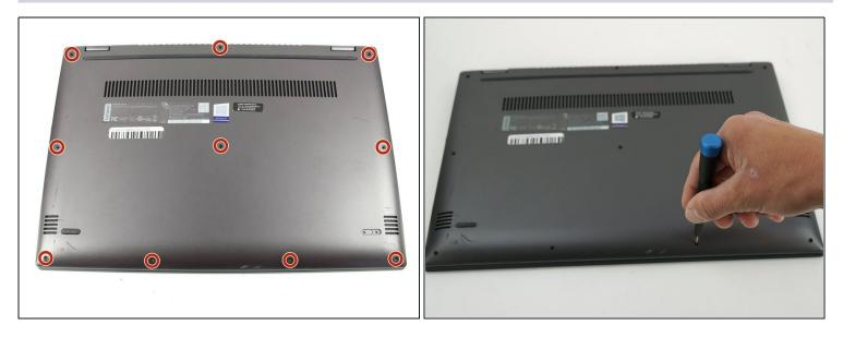
Remove the ten 5 mm Phillips #00 screws that are holding the back panel on.
