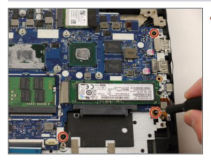
Using the Phillips #00 screwdriver, remove the three 5 mm Phillips #00 screws securing the motherboard.
