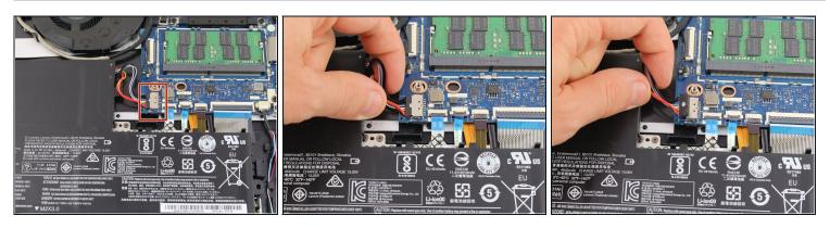
• Using your fingers, grasp the entire bundle of wires to pull the battery cable from its connector. This will cut off power to the motherboard.
