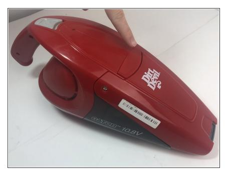
Press the button on the middle of the vacuum by pushing down on it and pulling the device apart.
