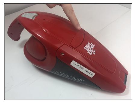
Press the button found at the top of the vacuum to separate the suction cup and the motor halves.
