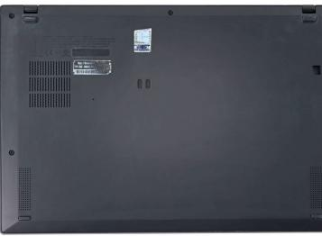
Use a Phillips #1 screwdriver to loosen the five captive screws securing the back cover.
