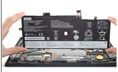
• Lift the battery straight out of its recess and remove it.
