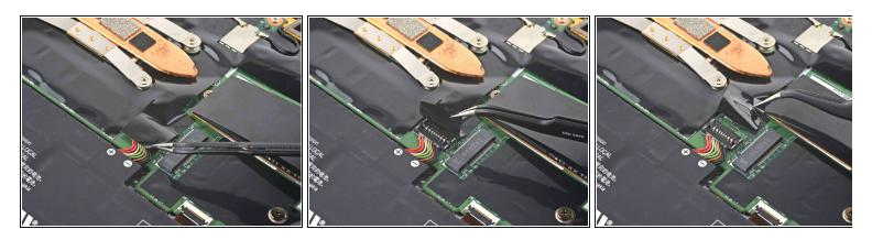
• Use tweezers or your fingers to peel back the plastic shield covering the battery connector.
