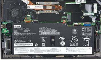
• Use a Phillips #0 screwdriver to remove the six 4.9 mm-long screws securing the battery.
