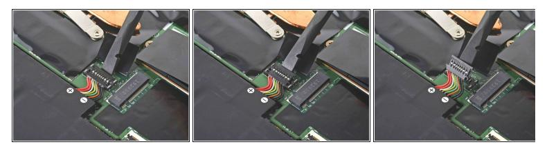
• Use the flat end of a spudger to pry up on and disconnect the battery cable.
