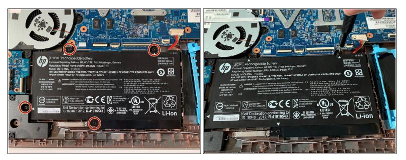
Using the Phillips #1 screwdriver, unscrew the four 6 mm screws.
