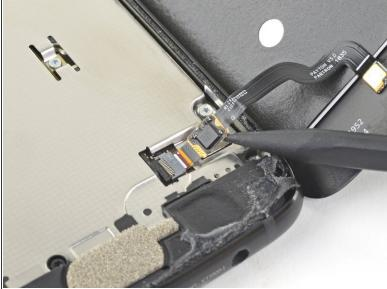
Slide the point of a spudger underneath the fingerprint sensor cable and gently pry up to loosen the cable from the phone.
