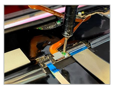
Lift the base off gently but don't pull too far - the battery is glued to the baseplate and the cable is screwed down to the motherboard! Use a T2 bit to remove the green screw and lift off the metal clasp, then unfasten the press-in battery connector.
