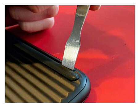
Use a metal spudger to gently lift up one corner of the rubber strips on the base. The strips are actually composed partially of hard plastic and will not stretch or deform, and should easily pop off with only gentle tugging.
