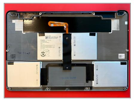
The inside of the baseplate with the glued-on battery and cable. No other components are attached to the baseplate.
