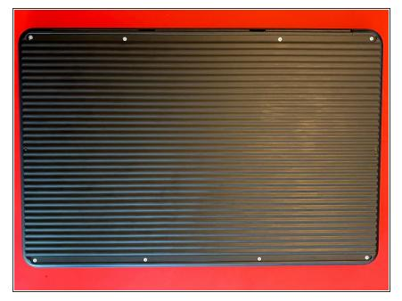
Now you can remove the ten T5 screws from the base. Keep track of the two screws from the centre front (by the touchpad) - they're ever so slightly shorter than the rest!
