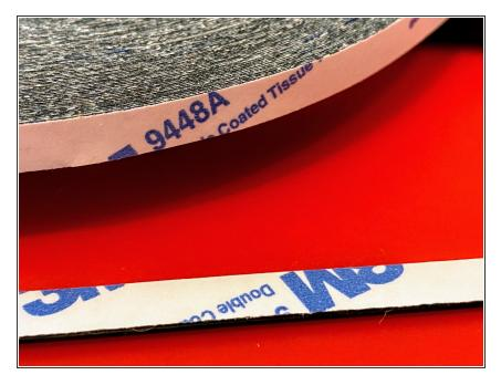
The adhesive on the strips doesn't feel very tacky after removal, so you may want to add a layer of 3M 9448A "double-coated tissue tape" to hold them on securely.
